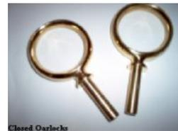
**c. "Davis Oarlock" Oarlock & Socket Combination** - Option A: 2" ID with 1-3/4" at gap. Socket plate 3-1/4" x 7/8", four fastener holes, Brass (Item **B21a**). Option B: 2"-1/4" with 2" at gap. Socket plate 3" x 1". Bronze (Item **B21b**).
