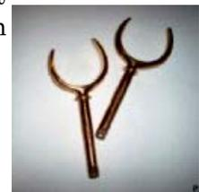
**d. English Open Oarlock Precision** machined in bronze with a higher arm facing forward to retain the oar and allow for maximum pull. Shank 1/2" x 4" with ID opening 2-1/2" and 2" at gap. (Item **B22**). Sockets see items **B14** and **B16**
